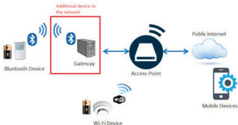
Figure 3 – You can use AA battery operated devices with ultra-low-power Wi-Fi
